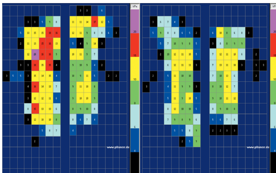
FIGURE 2. Images from a saddle pressure mat showing pressure scans of the same horse, saddle, and rider at the time of maximal force in the trot stride. The pommel is toward the top of the images, and the cantle is toward the bottom. The color bars on the right side of each scan show the colors used to represent increasing levels of pressure, from black (lowest) to pink (highest). The scan on the left shows the saddle without a pad; the scan on the right shows the effect of a sheepskin pad. Note that the sheepskin pad produces a more even pressure distribution, an overall reduction in peak pressures, and no pressures in the red or pink zones.
